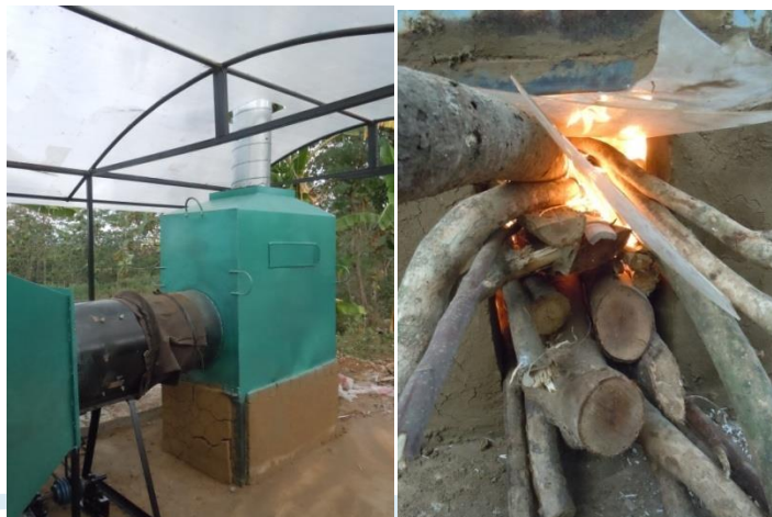
Fig. 5. Heat exchanger and furnace
